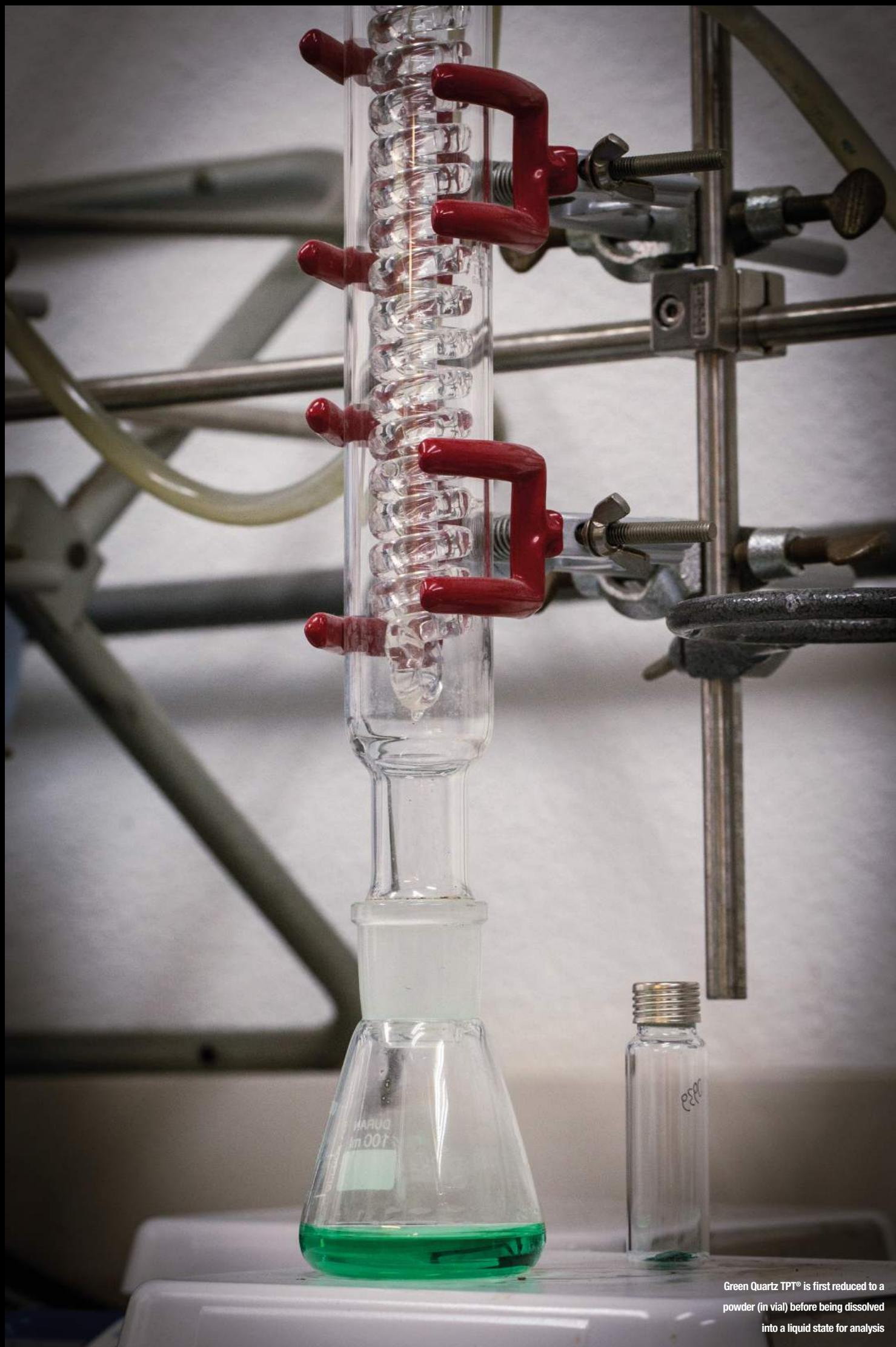
Green Quartz TPT® is first reduced to a powder (in vial) before being dissolved into a liquid state for analysis
